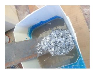
We put the mask on and throw the resin in the bucket, then, we start to throw chips until it has a medium saturation. Without saturating the chip mixture yet, we throw the catalyst.
